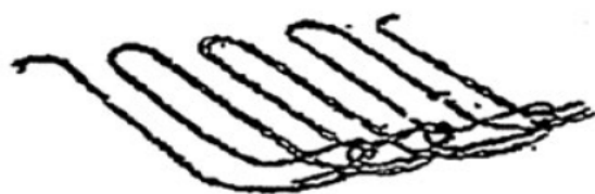
FIGURE 1. Catch cord diagram (Shuttleless construction)
